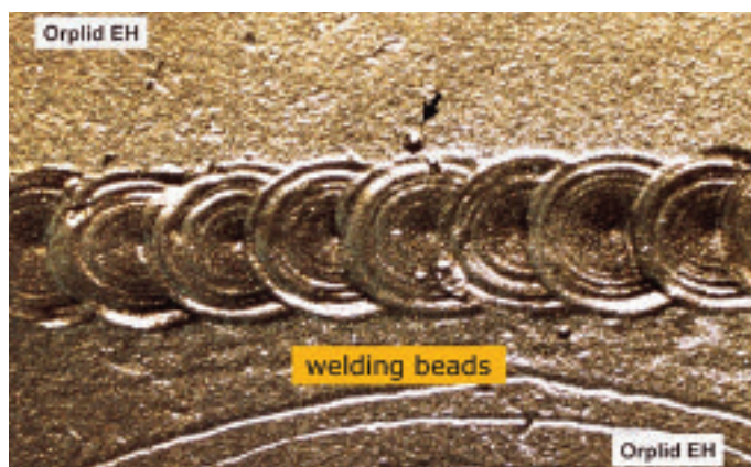
Fig. 1 Macroscopic view of the welding seam of a "homogenous" weld of a high-gold-content casting alloy (Orplid EH).
